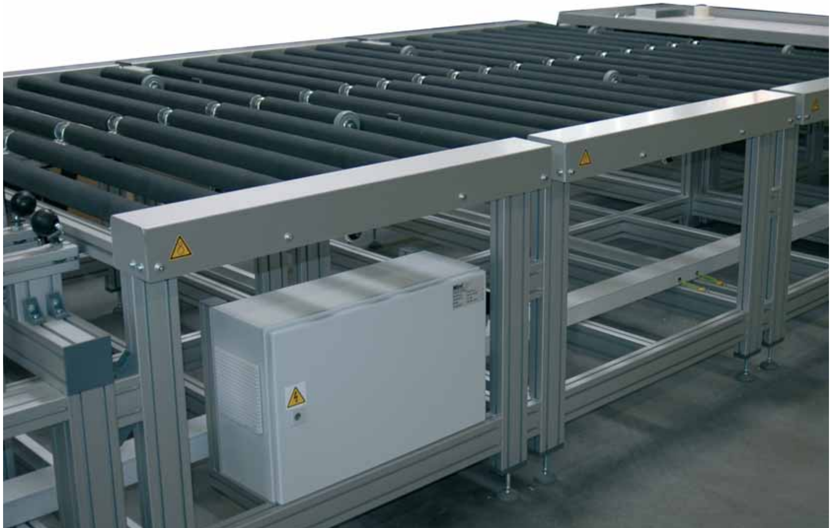
roller conveyor with mechanical accumulation protection
