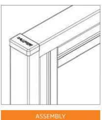
Simply push onto the end of the cable duct
