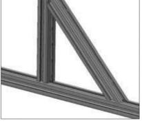
Screw on the profile groove of the frame construction with supplied hardware
